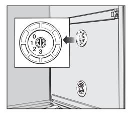
Use a coin or screwdriver to adjust the water hardness level selector in the wash cabinet. There is a click as each setting is reached.
